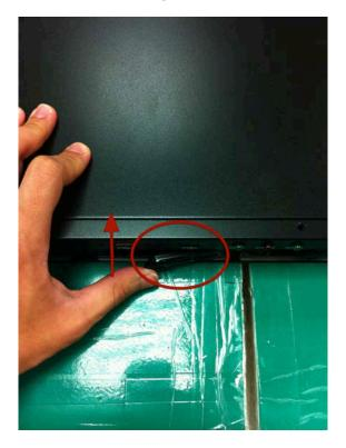
Secure the HDD tray by pushing in the latch, which locks the HDD tray with the unit.
